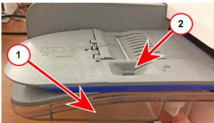
2. Add enough E-Z Seal® to bring the sealant level up to the bottom of the fill hole. Do not overfill your tank.
